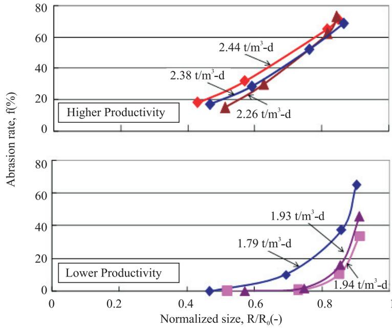
Fig.6. Coke abrasion rate (%) versus normalized coke size ( $R/R_0$ )(-) at various HM productivities.
