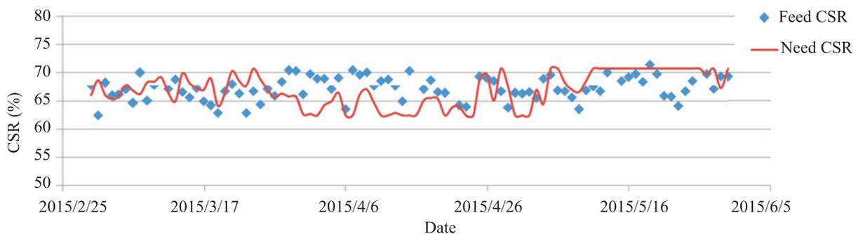
**Fig.10.** Comparison of daily CSR for feed coke in No. 3 BF and calculated CSR in this study during 2015/3-2015/5.
