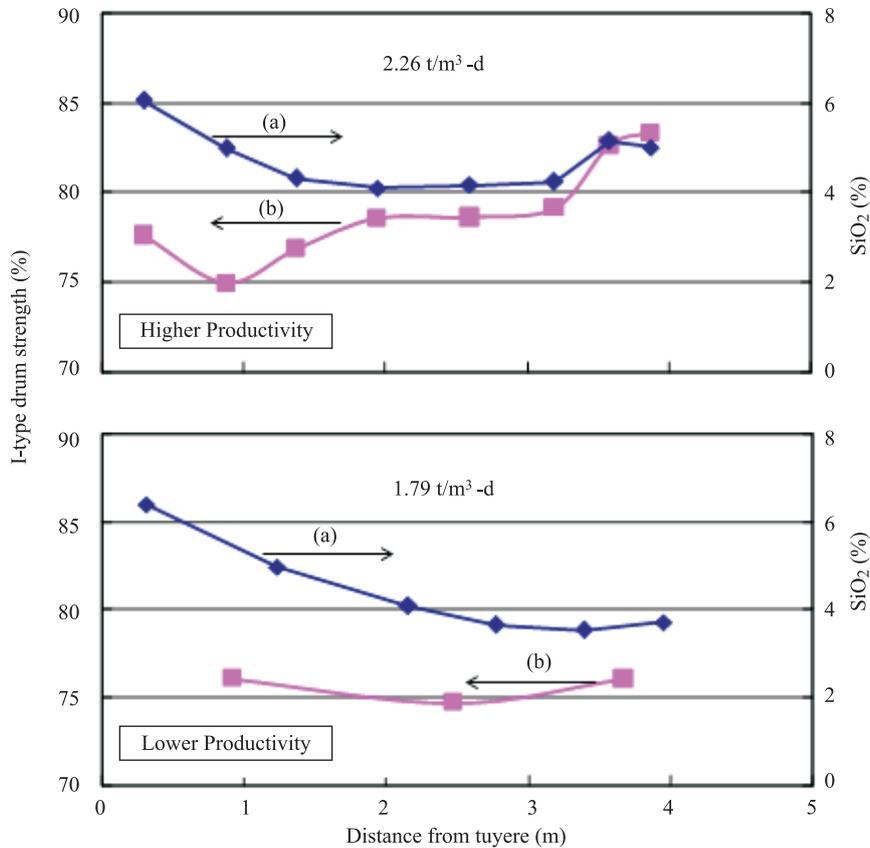
Fig.4. I-type drum strength of coke versus (a) SiO<sub>2</sub> content(%); (b) sampling distance from tuyere(m) at various HM productivities.
