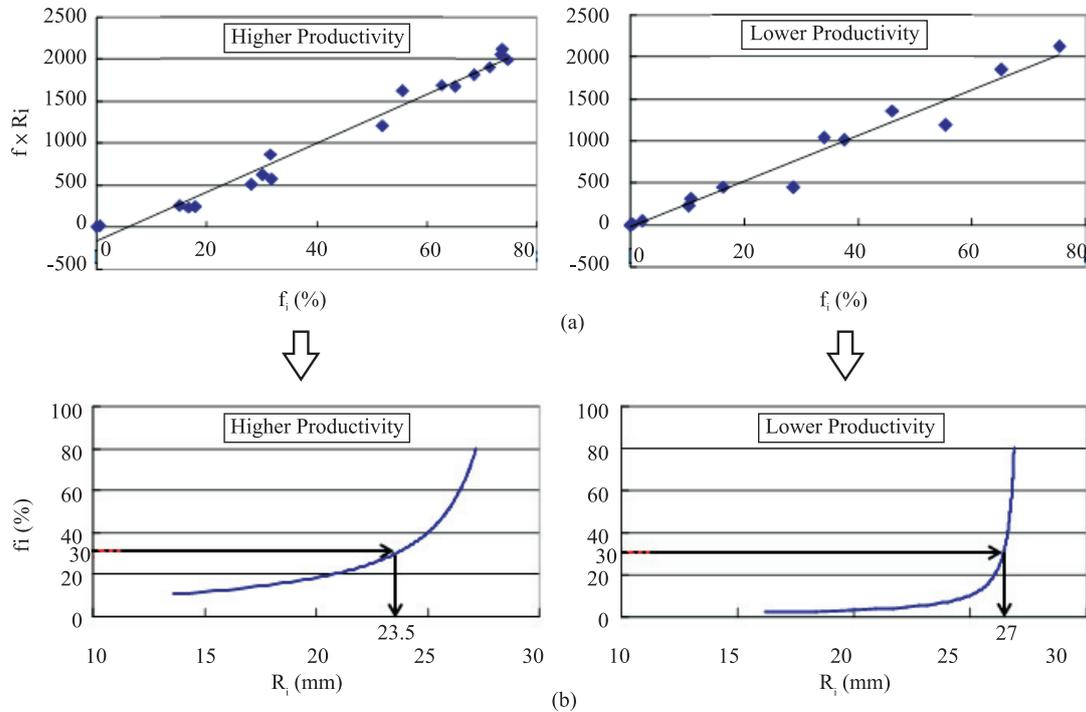
Fig.7. (a) [coke abrasion rate ( $f_i$ )  $\times$  coke radius ( $R_i$ )] versus coke abrasion rate ( $f_i$ ). (b) coke abrasion rate ( $f_i$ ) versus coke radius ( $R_i$ ) from equation (4) and (5).
