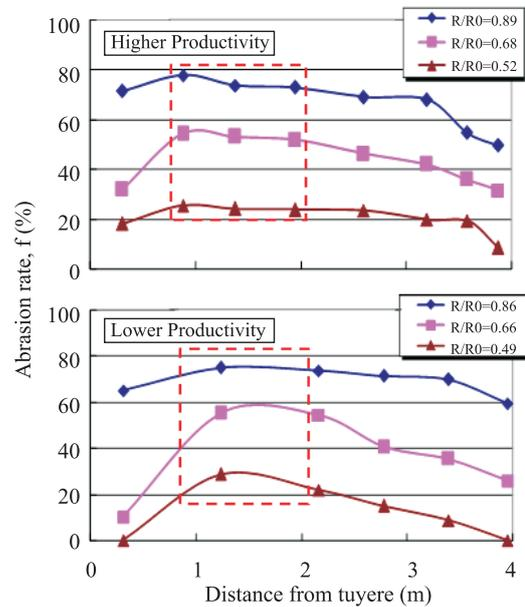
Fig.9. The coke abrasion rate (at various residual radius) versus sampling coke distance from tuyere at various productivities.
