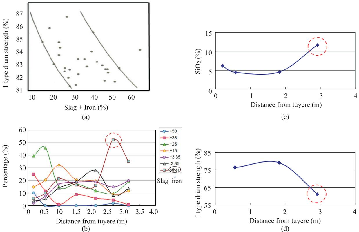
**Fig.5.** The effects of slag and iron on I-type drum strength of coke.
