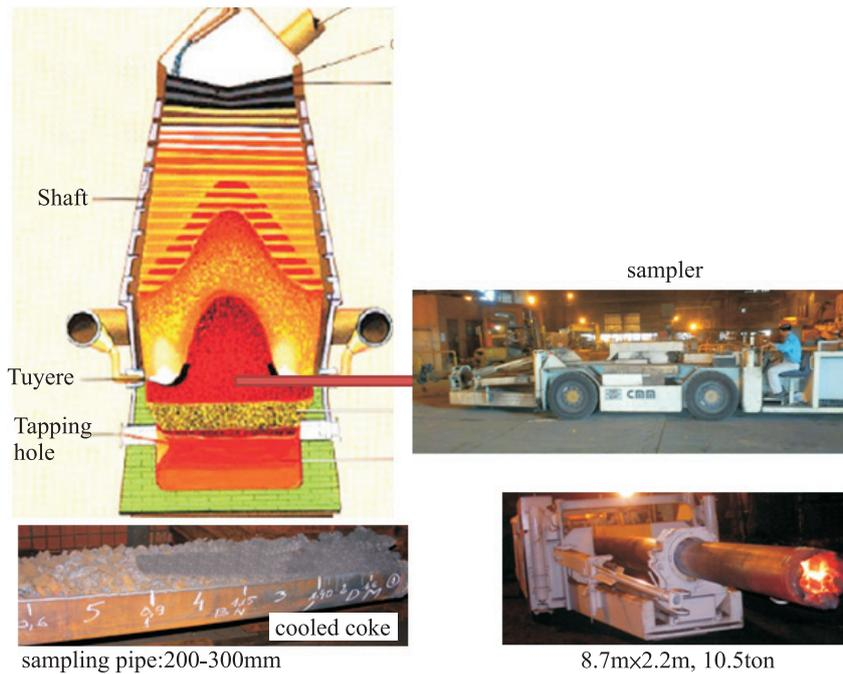
**Fig.1.** The Schematic diagram of high-temperature coke sampled from BF tuyere.
