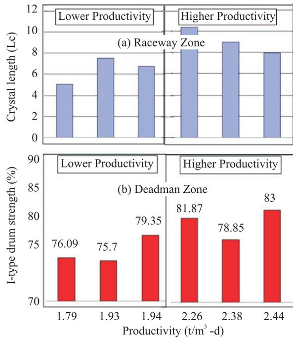
Fig.8. (a) Crystal length of raceway zone coke and (b) I-type drum strength of deadman zone versus HM productivities.
